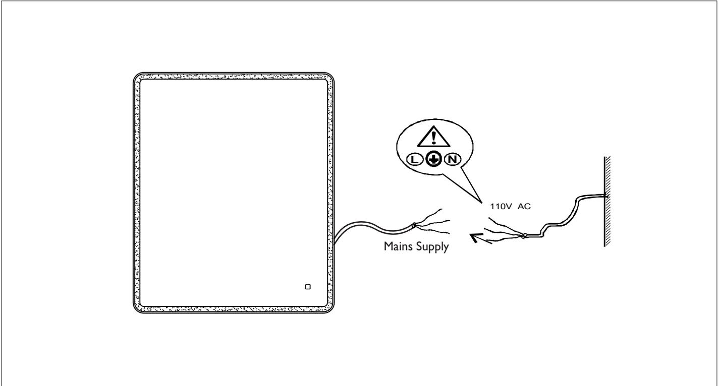
The next step is to make the electrical connection from the mirror to the main supply. Use the connection wire found at the rear of the mirror to make the necessary connections. A second person will need to hold the mirror in place whilst electrical connections are made.
